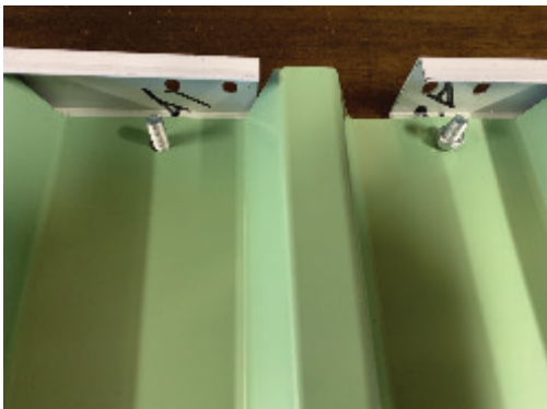
Figure 4. Connecting the long and short edge rails. These will end up at right angles to each other and be attached to the corner brackets as in Figure 7.
