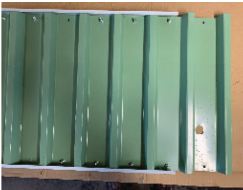
Figure 2. This shows the position to attach the panel with the hole for the overflow pipe.
